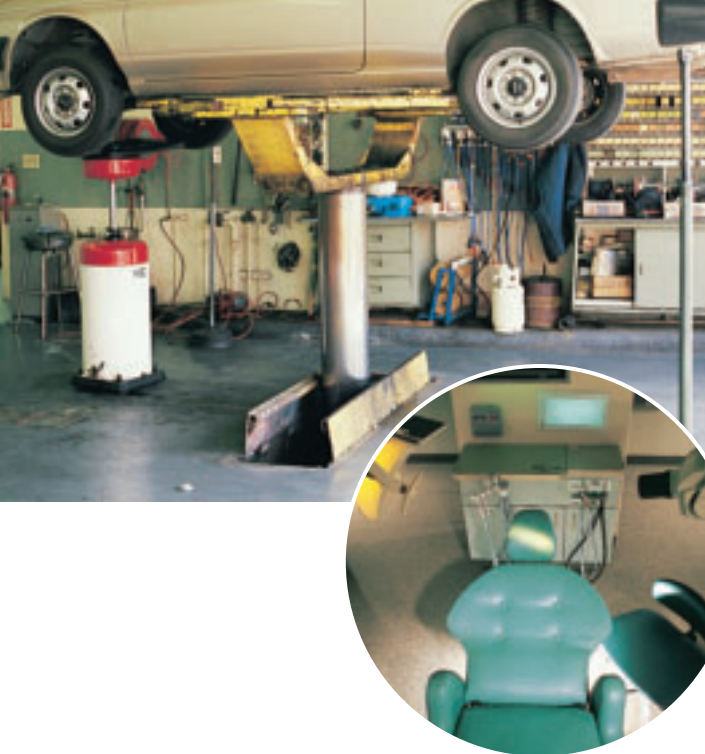
Figure 24 A hydraulic lift utilizes Pascal's principle to help lift this car and this dentist's chair.
